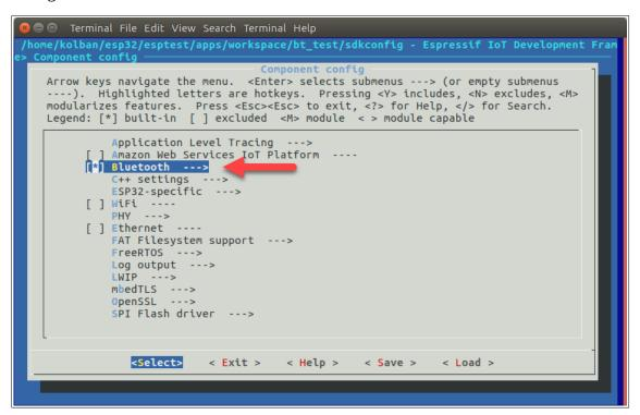
Next drill into the Bluetooth entry and ensure "Bluedroid Bluetooth stack enabled" is selected:
