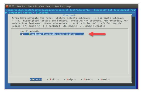
Finally, drill into the "Bluedroid Bluetooth stack enabled" and set the "Bluetooth event (callback to application) task stack size" to be 8000 (or more).
